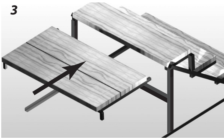
3 Slide the step platform into the sleeve on the step.
