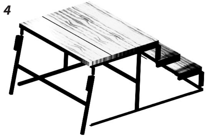
4 Insert "H" frame (B) into the back of the platform and rest "H" frame (B) on metal runner. (Handrail bracket to face out)
